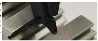
Gap/Step/Angle - As vehicles are assembled, the fit-up of various parts is inspected by measuring the width of the gap between two adjacent panels and the alignment of the two surfaces, also called flushness. Today's vehicles are designed with flowing contours, angled panels, edges with large radii and closure seals in the gaps. Mechanical devices struggle to measure gap and flush features on such complex surfaces. LaserGauge @ can help!
