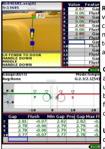
**Routine Mode** – Routine mode allows the user to run inspection routines developed using the LGWorks software. Multiple routines can be stored on the controller and automatically opened with the entry of an associated VIN, trace number or other identifier. Graphical and text instructions guide the operator to the proper measurement locations. Color-coded results and audible tones alert the operator to out-of-spec conditions.
