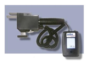
The plastic coated fingers create a non-marring version that prevents the operator or sensor from producing scratches. The handle grip can be attached in 2 different positions for optimum use at the different locations like on rear deck lid or sun roof. The system will capture the maximum (peak) force created by the automatic window drive before the safety mode returns the motion.
