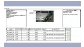
Data Files – Data files are formatted by the user and can vary by routine. The user has a choice of delimiters and the file can include information contained in the routine or found on the controller. Operator input fields and LaserGauge® generated information can also be included in the data file, such as date, time, shift, operator, VIN, feature label, description, etc.
