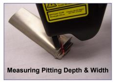
**Scanning Resolution** – With a 0.250" field-of-view (FOV), the HS410 has a horizontal scanning resolution of 0.0005". The vertical or depth accuracy is  $\pm$  0.00025" (6mm).
