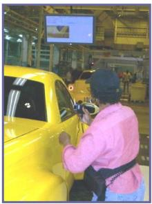
**Inspection Routines** - The LGWorks Run-Time software sends commands through the RF transceiver to the LG4101, giving it the set-up information needed for each measurement in the inspection routine. Commands to the LaserGauge® system include messaging displayed on the sensor LCD and the virtual gauge settings used to make a measurement. As measurements are taken, results are sent back to the computer to be displayed on the monitor and saved to a data file.
