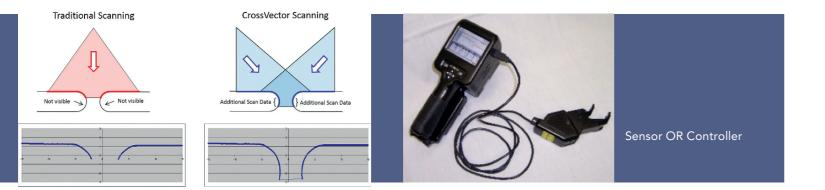
DSP Cross-Vector Sensor. Or if the user chooses, a LaserGauge USB sensor (such as the TS800) can be plugged into the HS763 USB port and the sensor then becomes a controller. The 3.5" color display of the sensor will broadcast the profile and data table as the USB sensor is triggered. Data and scans are saved to the sensor as if using a standard controller.
