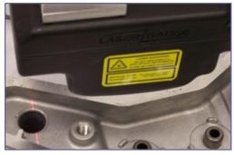
**Standoffs** - Since mechanical standoffs are used only to bring the sensor into an optimal depth-of-focus position, standoffs are not necessary for applications where the sensor is mounted to a fixture or robot. Positioning the sensor at the optimum distance from the part can be designed into the fixture or can be controlled robotically with feedback from the scan.
